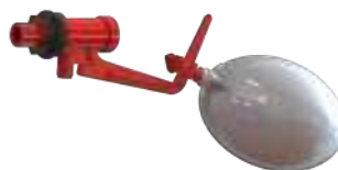
4204R Float for intensive rearing. Meets the need for high-pressure water capacity. The ø6mm nozzle allows perfect operation up to a maximum pressure of 5bar
