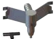
**9002** Drip drinker with stainless steel elastic connection, connectable with ø9mm flex pipe art. 9101. The tank should be positioned 20 cm higher. The ideal position is 25 cm from the bottom of the cage.
